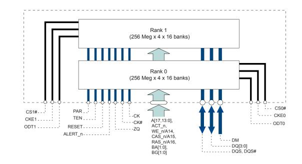
Figure 1: Functional Block Diagram (256 Meg x 4 x 16 Banks x 2 Ranks)
