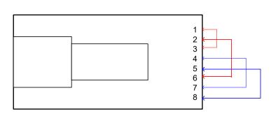
The external loopback test setup requires the presence of a MAC that will originate the frames to be sent out through the PHY. Instead of a normal RJ-45 cable, the loopback stubs allows the PHY to self-link at 1000 Mbps. It also allows the actual external loopback. See Figure 25. The MAC should see the same packets it sent, looped back to it.
