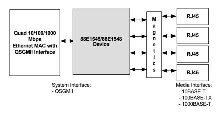
Figure 2: 88E1543/88E1548 Device Application - SGMII (System) to Copper
