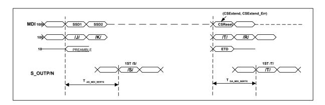
1. 10/100/1000BASE-T to SGMII latency timing (Register 27\_4.14 = 1) only applies when QSGMII crossover loopback is enabled.
