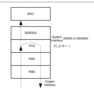
Figure 21: Copper Line Loopback Data Path
