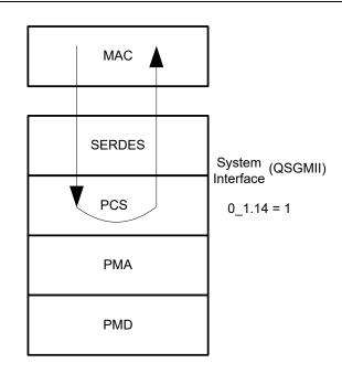
Figure 18: System Interface Loopback Diagram - Fiber Media Interface
