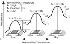
The temperature of the resistor will increase the same  $\ensuremath{ \ensuremath{ \square } } T$  from the standard terminal part temperature regardlless of the ambient temperature when the same power is applied. This is because there is hardly any heat dissipation from the resistor surface to the ambient air.
