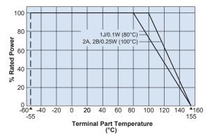
For resistors operated at a terminal part temperature of described for each size or above, a power rating shall be derated in accordance with the above derating curve.
