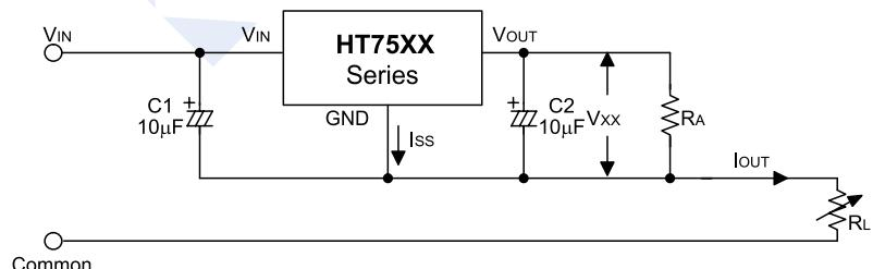
$$I_{OUT} = \frac{V_{xx}}{R_A} + I_{ss}$$
