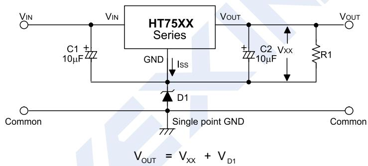
$$V_{OUT} = V_{xx} + V_{D1}$$
