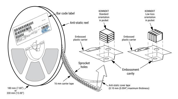
Table 4 - Carrier Tape Configuration, Embossed Plastic (mm)
