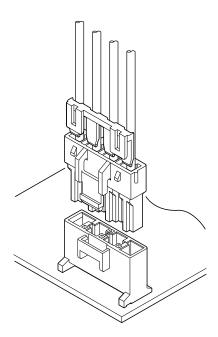
This VYH connector is designed for wire-toboard 6.5 mm pitch connector corresponding to large current. Secondary retainer, which prevents from insufficient insertion of contact and coming off contact, may use and large current circuit can be connected certainly and safely.
