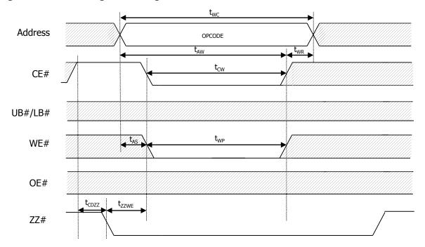
Figure 12: DPD Entry and Exit Timing
