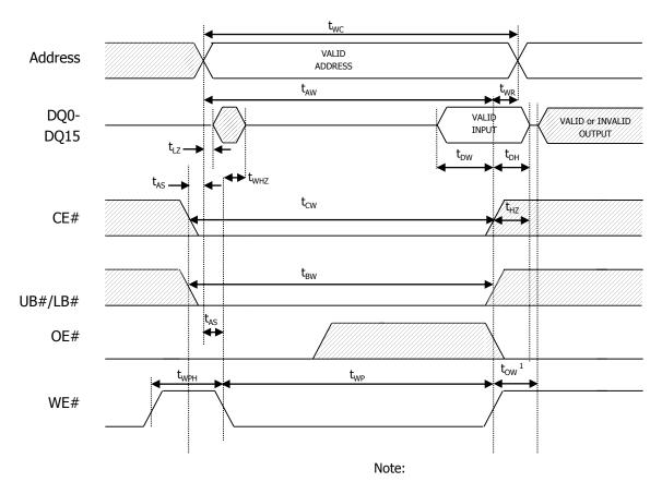
1.  $t_{DH}$  shouldn't be longer than  $t_{OW}$  when End of Write changes operating mode into READ.
