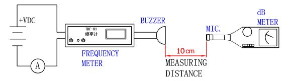
In the measuring test, buzzer is placed as follows:
