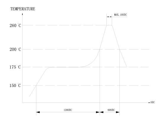
Heat resistant line (Used when heat resistant reliability test is performed) (2)Manual soldering
