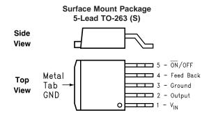
Order Number LM2592HVS-3.3, LM2592HVS-5.0, or LM2592HVS-ADJ
