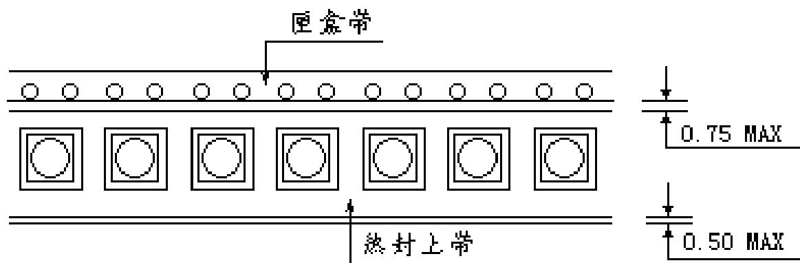
Deviation between carrier tape and seal tape shall be less than 0.5mm
