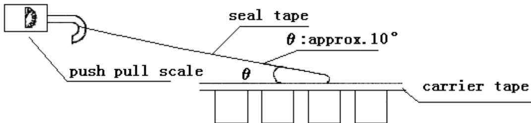
Reasonable pulling strength: 0.092~0.882N; Pulling speed: 200~300mm/min.
