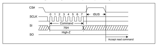
Figure 30. Program/Erase Suspend Sequence Diagram
