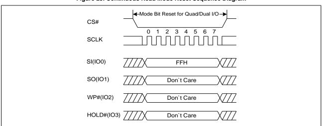
Figure 29. Continuous Read Mode Reset Sequence Diagram
