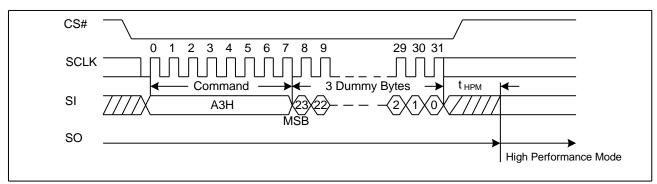
Figure 27. High Performance Mode Sequence Diagram
