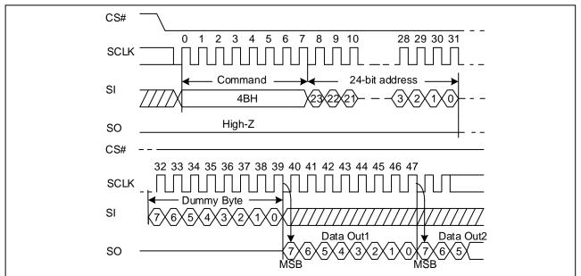
Figure 28. Read Unique ID Sequence Diagram
