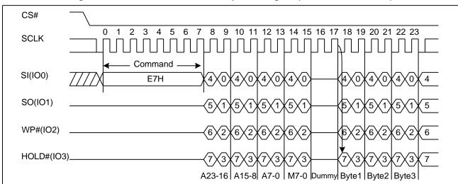
Figure 13. Quad I/O Word Fast Read Sequence Diagram (M7-0= 0XH or not AXH)
