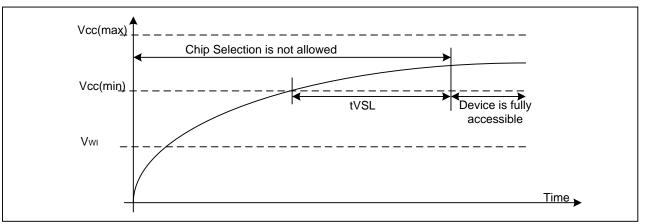
Table6. Power-Up Timing and Write Inhibit Threshold
