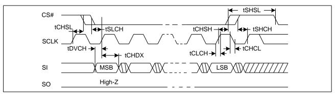
Figure 41. Output Timing
