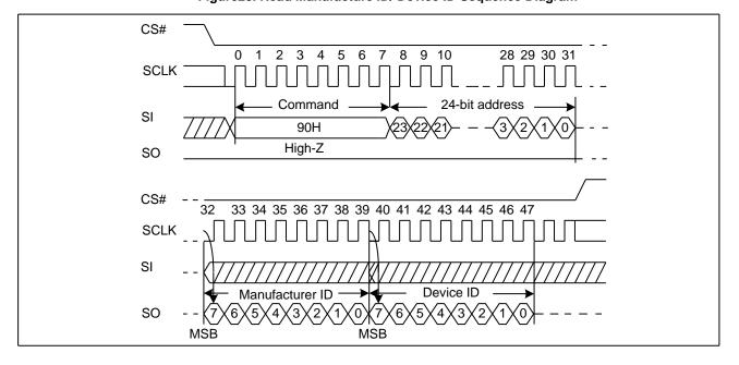
Figure 25. Read Manufacture ID/ Device ID Sequence Diagram
