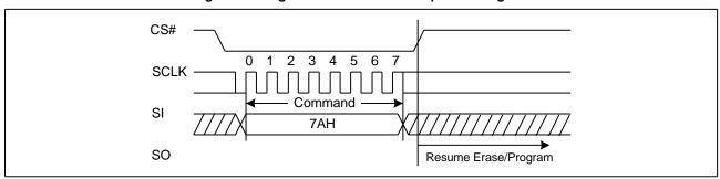
Figure 30. Program/Erase Resume Sequence Diagram
