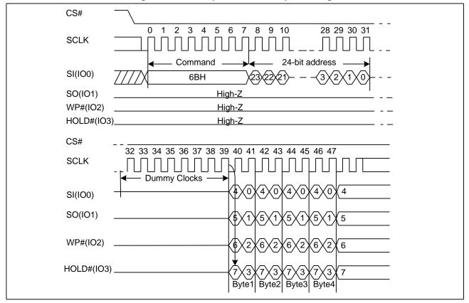
Figure 11. Quad Output Fast Read Sequence Diagram
