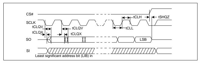
Figure 47. Resume to Suspend Timing Diagram
