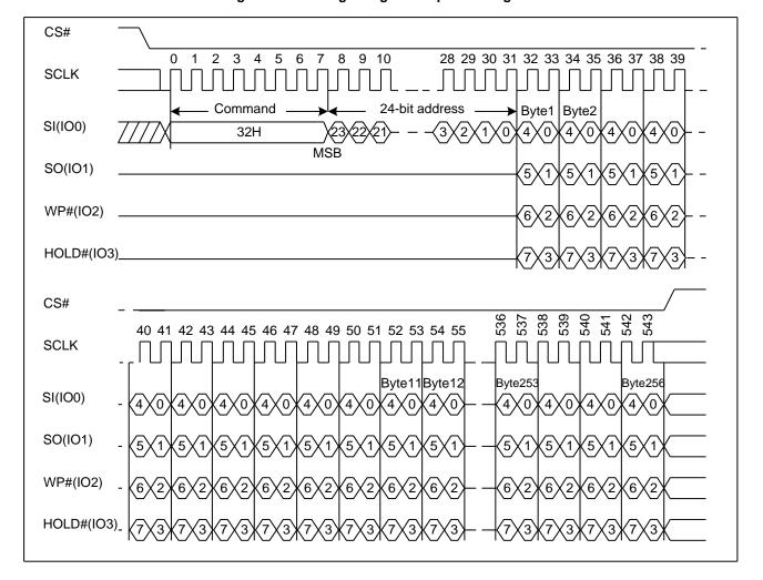
Figure 17. Quad Page Program Sequence Diagram
