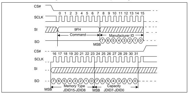
Figure 28. Read Identification ID Sequence Diagram
