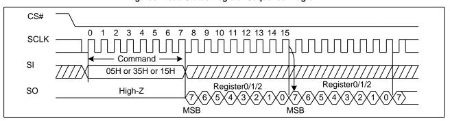
Figure 6. Read Status Register Sequence Diagram
