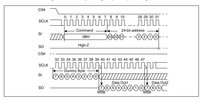
Figure 9. Read Data Bytes at Higher Speed Sequence Diagram
