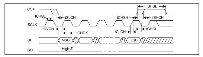
Figure 46. Output Timing
