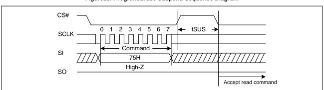
Figure 29. Program/Erase Suspend Sequence Diagram
