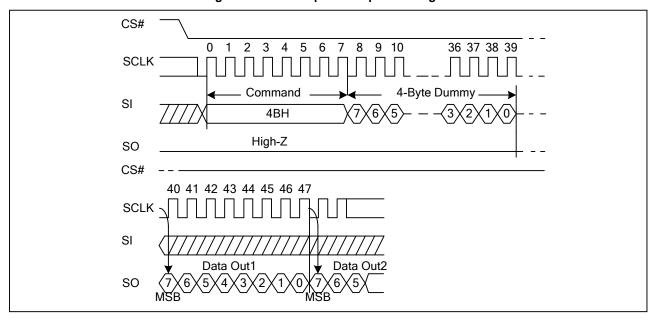
Figure 40 Read Unique ID Sequence Diagram
