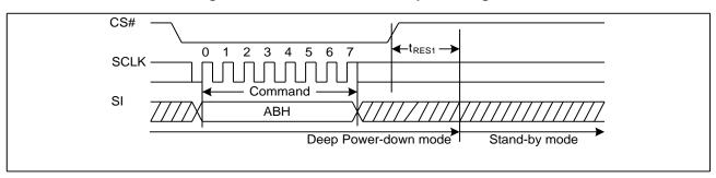
Figure 23. Release Power-Down Sequence Diagram
