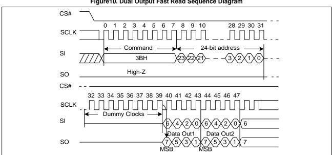
Figure 10. Dual Output Fast Read Sequence Diagram
