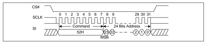
Figure 19. 32KB Block Erase Sequence Diagram
