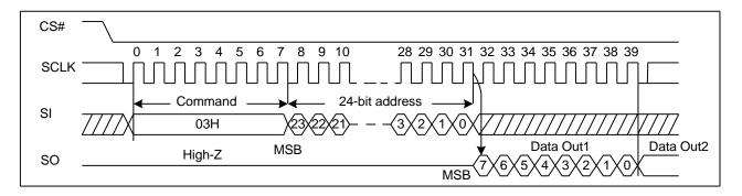
Figure 7. Read Data Bytes Sequence Diagram
