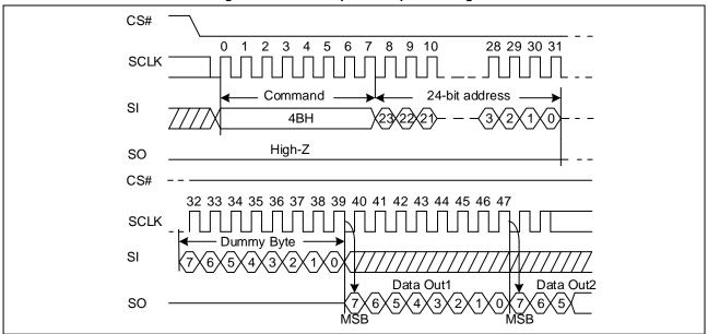
Figure 30. Read Unique ID Sequence Diagram
