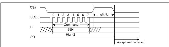
Figure 31. Program/Erase Suspend Sequence Diagram
