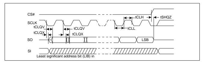
Figure 43. Resume to Suspend Timing Diagram
