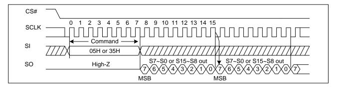
Figure 5. Read Status Register Sequence Diagram
