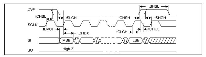
Figure 42. Output Timing
