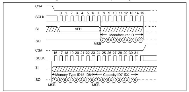
Figure 29. Read Identification ID Sequence Diagram
