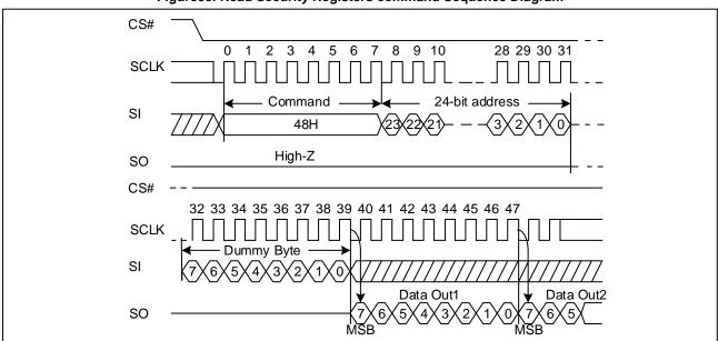
Figure 35. Read Security Registers command Sequence Diagram
