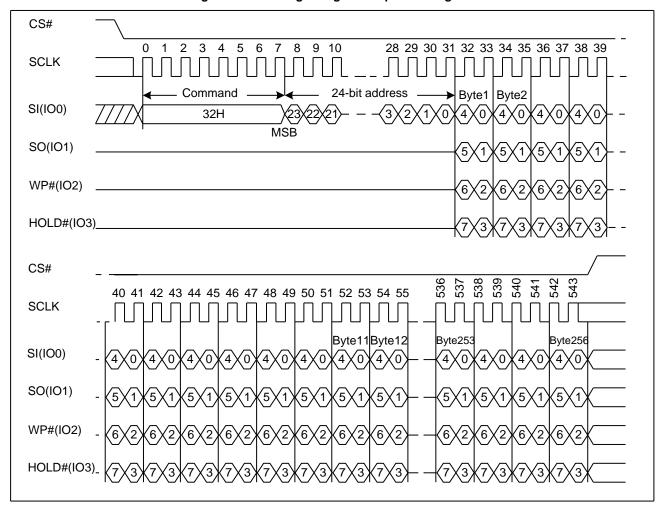
Figure 17. Quad Page Program Sequence Diagram
