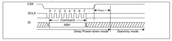
Figure 25. Release Power-Down/Read Device ID Sequence Diagram
