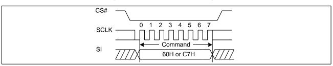
Figure 21. Chip Erase Sequence Diagram
