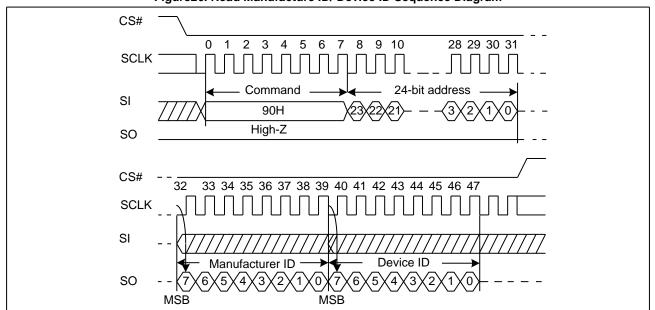
Figure 26. Read Manufacture ID/ Device ID Sequence Diagram
