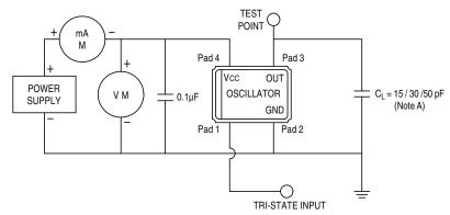
Note A: CL includes probe and fixture capacitance 15 pF S1700 to 80 MHz 15pF S1703 to 64 MHz (30pF to 80MHz) 50 pF S1750 to 67 MHz
