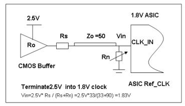
$Rs = 33\Omega$  with  $Rn = 100\Omega$  to transition 3.3V CMOS to 2.5V Rs=  $43\Omega$  with Rn =70 $\Omega$  to transition 3.3V CMOS to 1.8V
