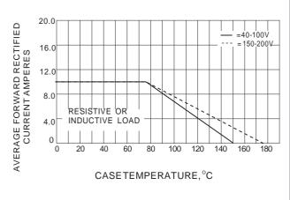
Fig.1 - FORWARD CURRENT DERATING CURVE
