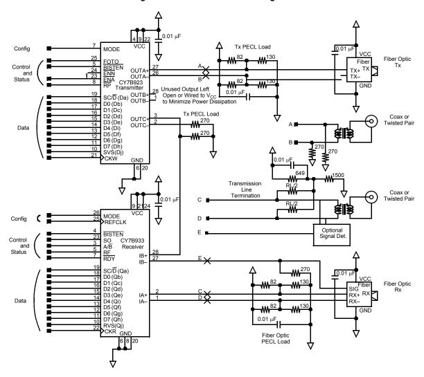
Figure 7. HOTLink Connection Diagram
