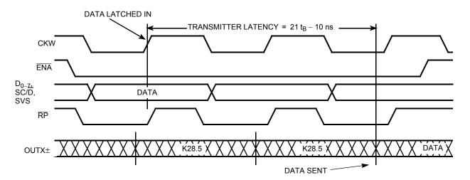
Figure 12. CY7B923 Transmitter Data Pipeline
