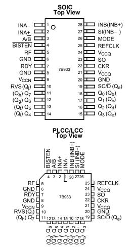
Figure 3. CY7B933 Receiver Pin Configurations
