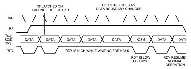
The transmitter and receiver parallel interface timing and functionality can be made to match the timing and functionality of either an asynchronous FIFO or a clocked FIFO by appropriately connecting signals (see Figure 6 on page 12). Proper operation of the FIFO interface depends upon various FIFO-specific access and response specifications.
