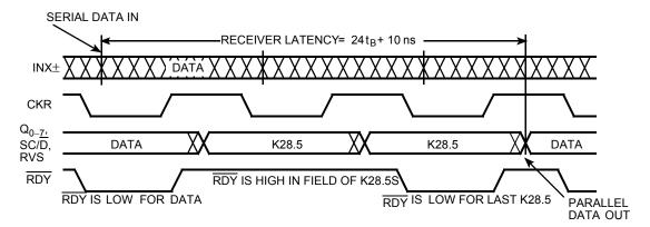
Figure 4. CY7B933 Receiver Data Pipeline in Encoded Mode
