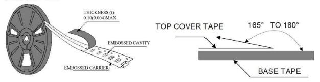
The force for peeling off cover tape is 30 to 100 grams in to arrow direction.
