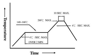
3. DIP soldering (Wave Soldering):
