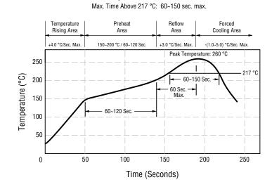
Peak Temperature: 260 °C max. Max. Peak Temperature -5 °C: 30 sec. max.
