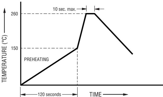
Wave soldering is suitable for 2410 size models.
