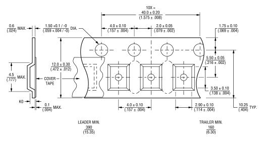
K0  $\frac{0.65 \pm 0.10}{(.026 \pm .004)} \text{ MF-USML175/6} \sim \text{MF-USML260/6, MF-USML175/12} \sim \text{MF-USML260/12}$   $\frac{1.10 \pm 0.10}{0.026 \pm .004} \text{ MF-USML300/6} \sim \text{MF-USML700/6, MF-USML300/12} \sim \text{MF-USML550/12}$
