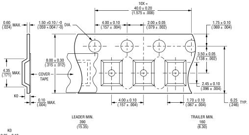
$\frac{0.95 \pm 0.10}{(.037 \pm .004)} \text{ MF-PSML075/6} \sim \text{MF-PSML175/6}, \text{ MF-PSML075/12} \sim \text{MF-PSML175/12}$
