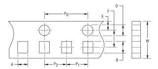
$\frac{40 \pm 0.2}{(1.575 \pm .008)}$ Accumulated dimensional tolerance
