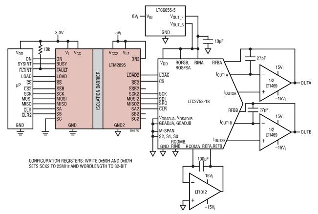
Figure 12. Isolated Dual-Channel 18-Bit DAC with Read Back
