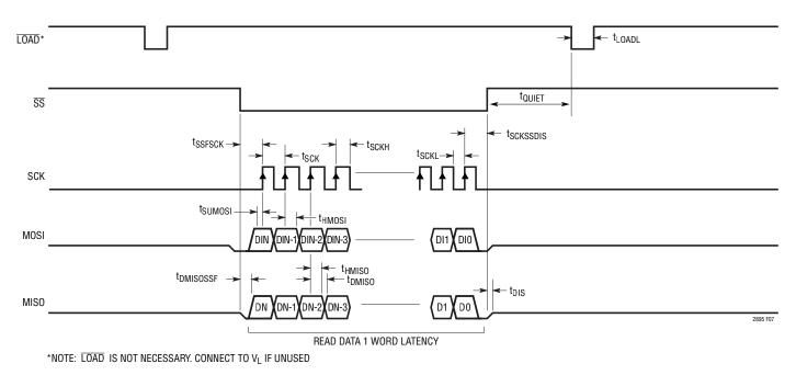
Figure 7. Logic Side Interface
