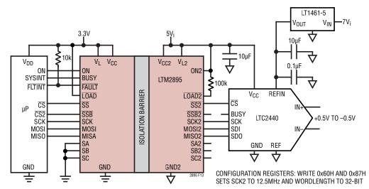
Figure 13. Isolated System Measurement with 24-Bit SDM ADC
