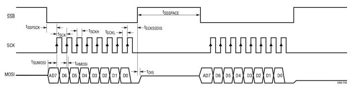
Figure 6. Writing Configuration Registers Timing Diagram
