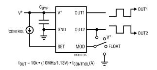
Figure 5. Current Controlled Oscillator
