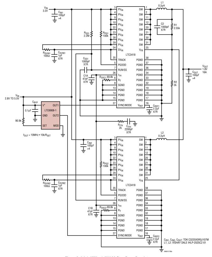
Figure 8. (a) 1.1MHz, 1.8V/16A Step-Down Regulator
