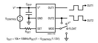
Figure 6. Voltage Controlled Oscillator
