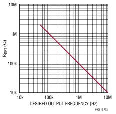
Figure 2. R<sub>SET</sub> vs Desired Output Frequency
