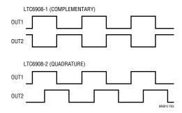
Figure 3. Output Waveforms for LTC6908-1, LTC6908-2
