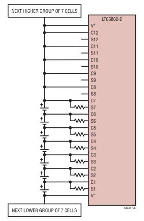
Figure 5. Monitoring 7 Cells with the LTC6802-2
