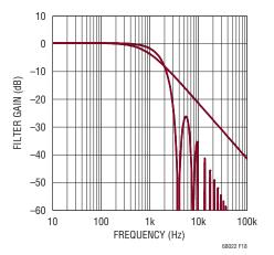
Figure 18. Noise Filtering of the LTC6802-2 ADC
