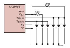
Figure 14. Using Diode Sensors as Hot-Spot Detectors
