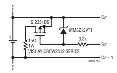
Figure 4. External Discharge FET Connection (One Cell Shown)
