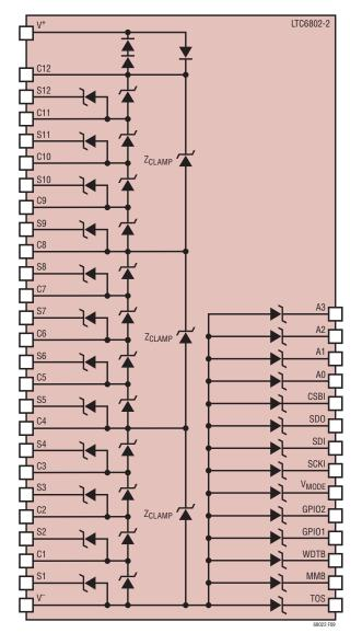
Figure 9. Internal Protection Diodes
