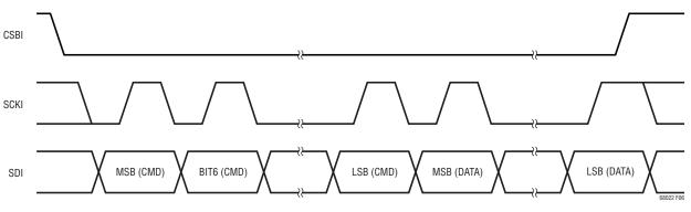
Figure 6. Transmission Format (Write)
