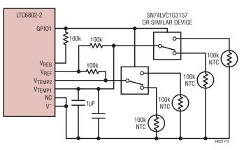
Figure 13. Expanding Sensor Count with Multiplexing
