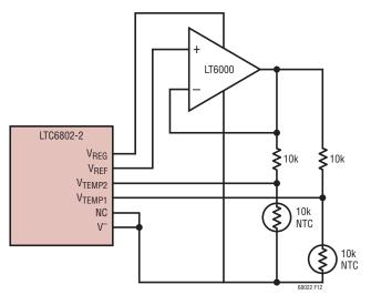
Figure 12. Buffering  $V_{REF}$  for Higher Current Sensors
