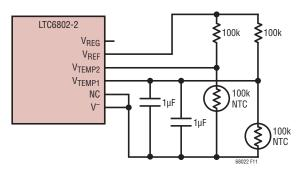
Figure 11. Driving Thermistors Directly from  $\ensuremath{\mathsf{V_{\text{REF}}}}$
