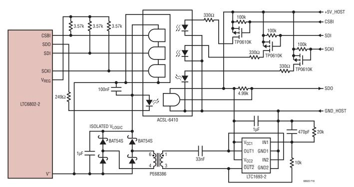
Figure 16. Providing an Isolated High-Speed Data Interface
