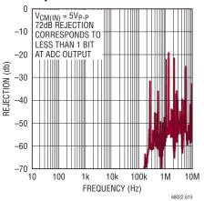
ADC Normal Mode Rejection vs Frequency
