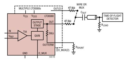
Figure 8. AC Coupled Output
