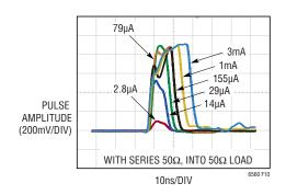
Figure 10. Output Pulse Over Input Current
