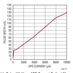
Figure 14. Pulse Width vs APD Current Optical Measurement
