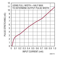
Figure 12. Pulse Stretching Detailed T = 25°C, Using FWHM
