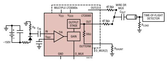
Figure 3. LTC6560 with AC Coupled Input and Output
