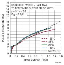
Pulse Stretching C<sub>IN</sub> = 2.0pF, Using FWHM
