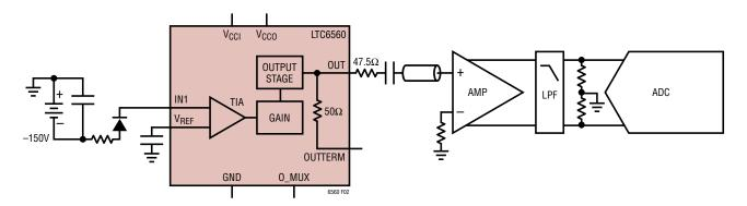
Figure 2. Typical Application with Output to an ADC
