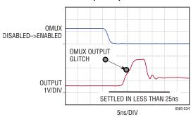
O\_MUX and Channel Switching Time for AC Coupled Input
