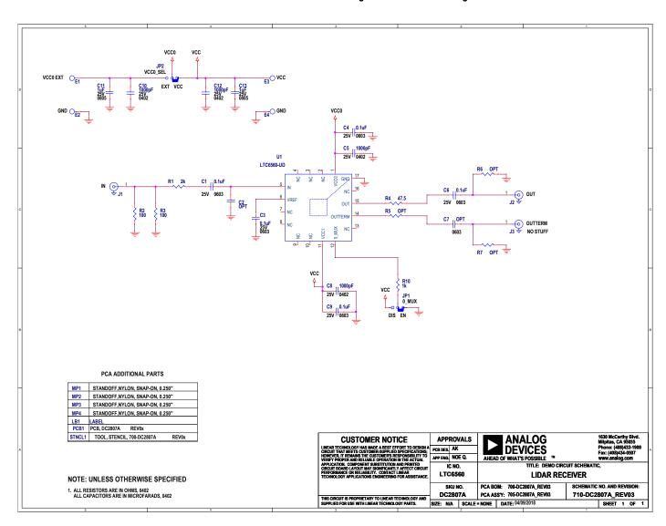
Evaluation board DC2803A allows for optical evaluation using a laser source. An onboard APD converts an optical pulse into a current pulse that is converted to an
