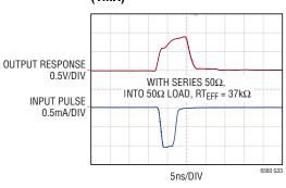
O\_MUX Switching Time DC Coupled Input
