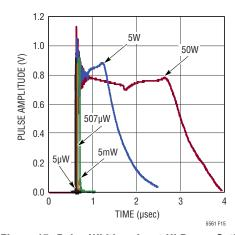
Figure 15. Pulse Width vs Input Hi Power Optical
