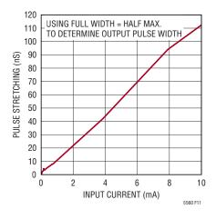
Figure 11. Pulse Stretching T = 25°C, Using FWHM
