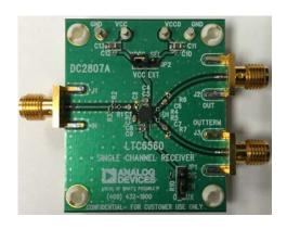
Figure 16. DC2807A Single Channel Electrical Evaluation Board
