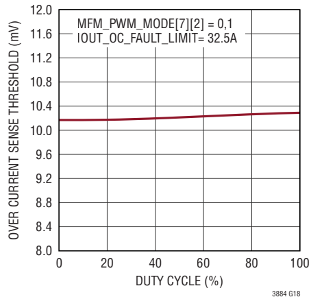
Current Sense Threshold vs Duty Cycle
