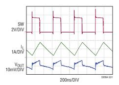
$3.3V_{\mbox{\footnotesize IN}}$  to  $1.2V_{\mbox{\footnotesize OUT}},$  2MHz TYPICAL APPLICATION  $I_{\mbox{\footnotesize LOAD}}$  = 1A
