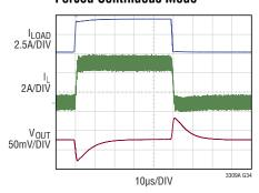
$3.3V_{IN}\;$  to  $1.2V_{OUT},\;2MHz\;TYPICAL\;APPLICATION\;C_{OUT}=66\mu F,\;L=220nH\;LOAD\;STEP:\;0.1A\;TO\;4.5A\;IN\;1\mu s$
