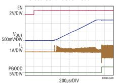
$3.3V_{\mbox{\footnotesize{IN}}}$  to  $1.2V_{\mbox{\footnotesize{OUT}}},$  2MHz TYPICAL APPLICATION  $R_{\mbox{\footnotesize{LOAD}}}=120\Omega$
