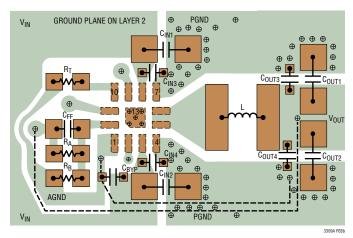
Figure 3b. Recommended PCB Layout for the LTC3309A with capacitors  $C_{OUT1}$  and  $C_{OUT2}$  rotated by 90°, which reduces high-frequency output ripple. Optional 0201 capacitors  $C_{OUT3}$  and  $C_{OUT4}$  further improve the high-frequency output ripple
