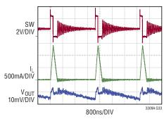
$3.3 V_{\mbox{\footnotesize{IN}}}$  to  $1.2 V_{\mbox{\footnotesize{OUT}}}, 2 \mbox{\footnotesize{MHz}}$  Typical application  $I_{\mbox{\footnotesize{LOAD}}} = 100 \mbox{\footnotesize{mA}}$
