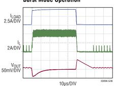
$3.3V_{IN}$  to  $1.2V_{OUT},$  2MHz TYPICAL APPLICATION  $C_{OUT}$  =  $66\mu F_{L}$  = 220nH LOAD STEP: 0.1A TO 4.5A IN  $1\mu s$
