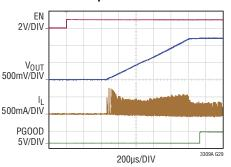
$3.3V_{IN}\,$  to  $1.2V_{OUT},\,2MHz$  TYPICAL APPLICATION  $R_{LOAD}$  =  $120\Omega$
