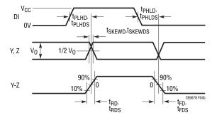
**Figure 4. Driver Timing Measurement**
