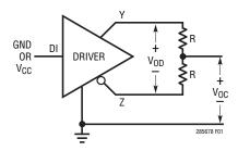
Figure 1. Driver DC Characteristics
