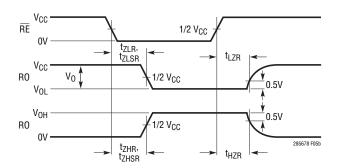
Figure 7. Receiver Enable/Disable Time Measurements
