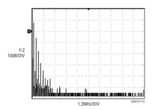
Figure 11. LTC2858-2 Driver Output at 100kHz Into 100 $\Omega$  Resistor
