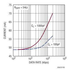
Figure 8. Supply Current vs Data Rate
