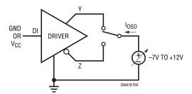
Figure 2. Driver Output Short-Circuit Current
