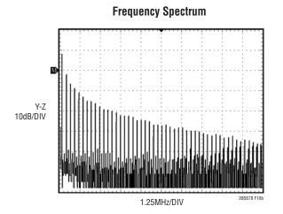
Figure 10. LTC2858-1 Driver Output at 100kHz Into 100 $\Omega$  Resistor
