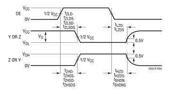
Figure 5. Driver Enable and Disable Timing Measurement
