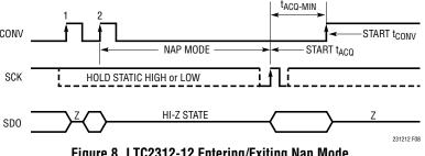
Figure 8. LTC2312-12 Entering/Exiting Nap Mode
