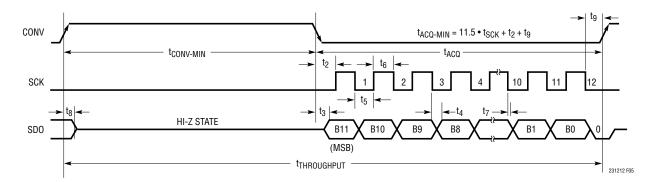
Figure 5. LTC2312-12 Serial Interface Timing Diagram (SCK Low During t<sub>CONV</sub>)
