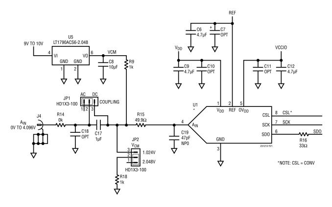
Figure 21. Partial 1563 Demo Board Schematic
