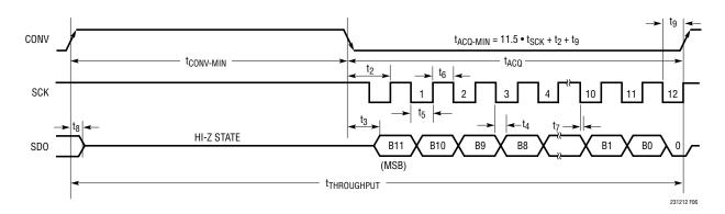
Figure 6. LTC2312-12 Serial Interface Timing Diagram (SCK High During t<sub>CONV</sub>)
