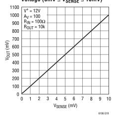
Output Voltage vs Input Sense Voltage ( $0mV \le V_{SENSE} \le 10mV$ )
