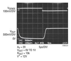
Step Response 50mV to 500mV ( $R_{IN} = 500\Omega$ )
