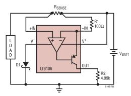
Figure 6. Schottky Diode Prevents Damage During Supply Reversal
