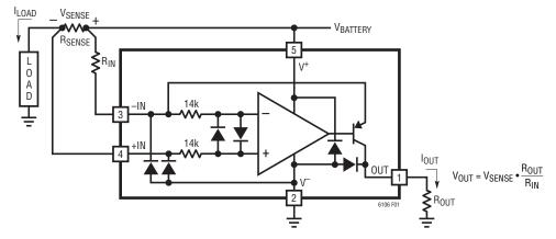
Figure 1. LT6106 Block Diagram and Typical Connection
