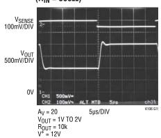
Step Response OmV to 50mV  $(R_{IN} = 500\Omega)$
