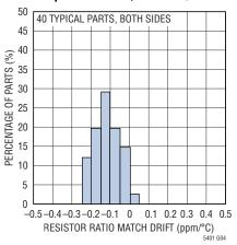
Resistor Ratio Matching Temperature Drift, G = 2V/V
