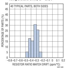
Resistor Ratio Matching Temperature Drift, G = 1V/V
