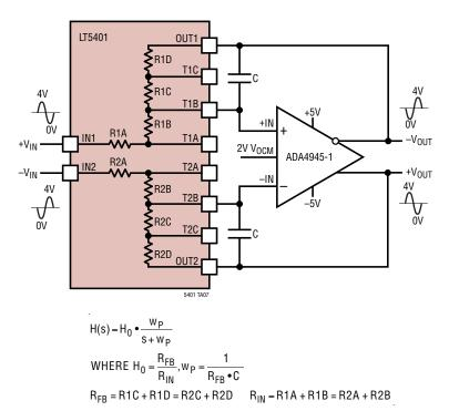
Precision Fully Differential Single Pole Low Pass Filter
