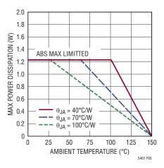
Figure 5. Safe Operating Area for Various  $\theta_{\text{JA}}$
