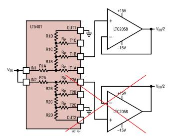
Figure 4. Voltage Divider
