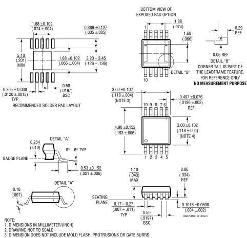
**MSE** Package 10-Lead Plastic MSOP, Exposed Die Pad (Reference LTC DWG # 05-08-1664 Rev I)
