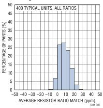
Resistor Ratio Matching Temperature Drift, G = 0.5V/V
