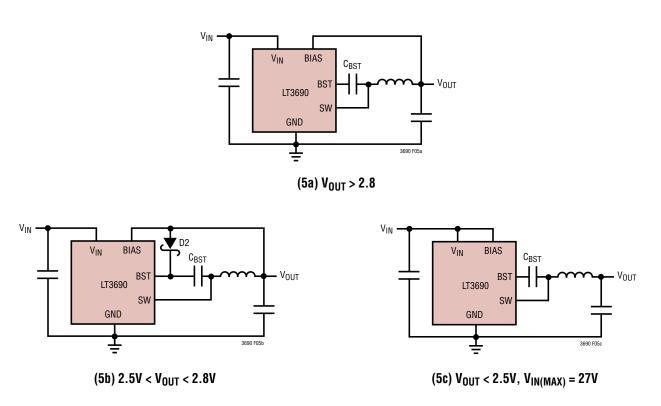
Figure 5. Three Circuits for Generating the Boost Voltage
