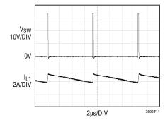
Figure 11. The LT3690 Reduces its Frequency to Below 250kHz to Protect Against Shorted Output with 36V Input
