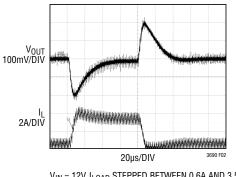
$V_{\text{IN}}$  = 12V,  $I_{\text{LOAD}}$  Stepped between 0.6A and 3.5A Front page application
