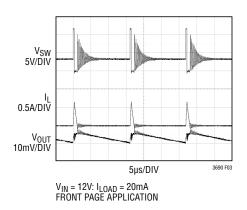
Figure 3. Burst Mode Operation
