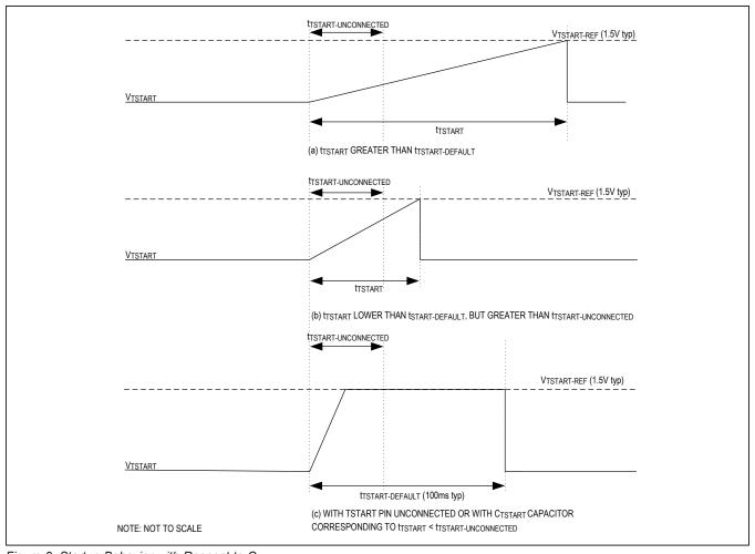
Figure 3. Startup Behavior with Respect to  $C_{TSTART}$
