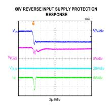
4.5V to 60V, 3A Current-Limiter with OV, UV and Reverse Protection
