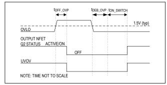
Figure 1. Overvoltage Fault Timing Diagram
