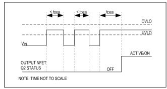
Figure 2. Debounce Timing Diagram
