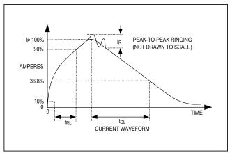
Figure 13. Human Body Current Waveform
