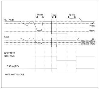
Figure 11. Fast Reverse Current Fault Timing Diagram
