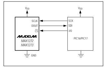
Figure 12. SPI Interface Connection for a PIC16/PIC17
