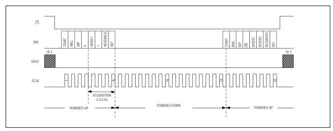
Figure 9. Immediate Power-Down Timing
