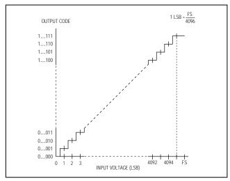
Figure 13a. Unipolar Transfer Function
