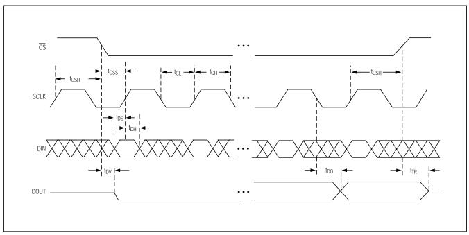
Figure 4. Detailed Serial Interface Timing
