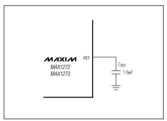
Figure 7a. Internal Reference Configuration
