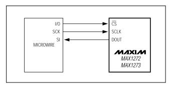
Figure 10b. MICROWIRE Connections
