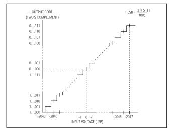
Figure 13b. Bipolar Transfer Function
