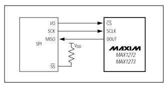
Figure 10a. SPI Connections
