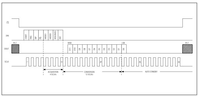
Figure 5. Conversion Timing, 21 Clocks/Conversion
