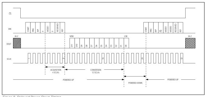
Figure 8. Delayed Power-Down Timing
