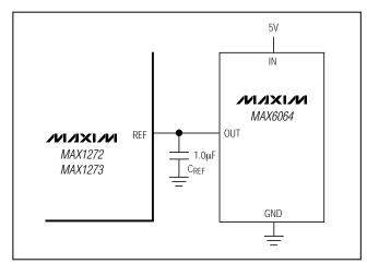
Figure 7b. External Reference Configuration
