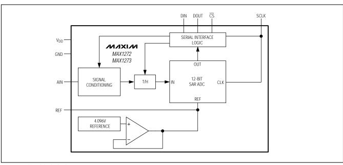
Figure 2. Simplified Block Diagram
