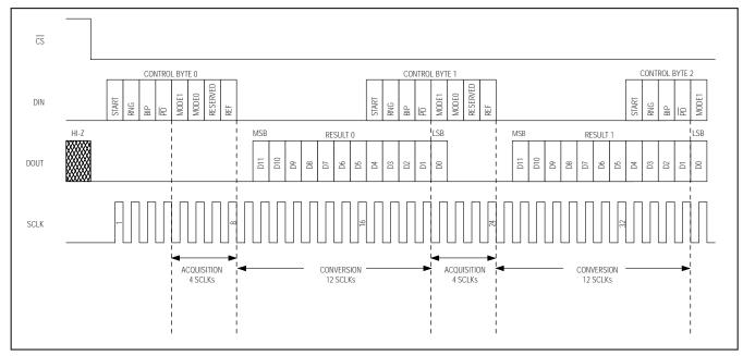
Figure 6. Conversion Timing, 16 Clocks/Conversion
