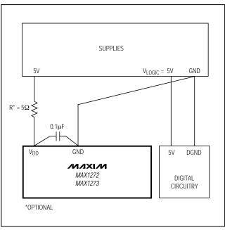
Figure 14. Power-Supply Grounding Connections
