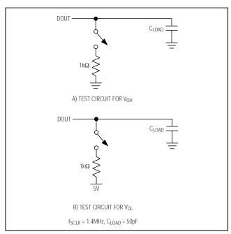
Figure 1. Output Load Circuit for Timing Characteristics
