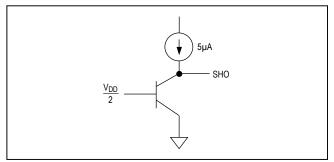
Figure 7. SHO Output Circuit
