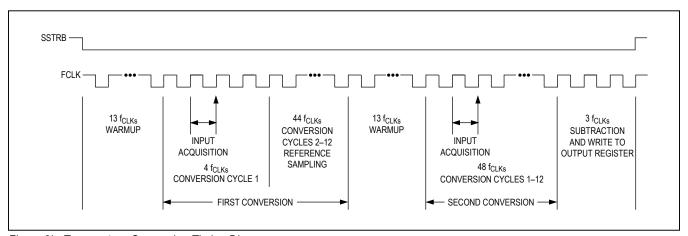
Figure 3b. Temperature Conversion Timing Diagram
