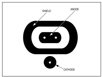
Figure 8. Remote Diode Shielding for PC Boards
