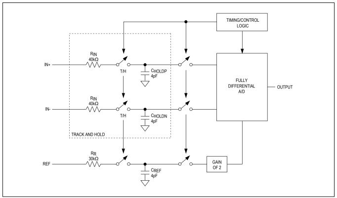
Figure 2. Converter Input Structure
