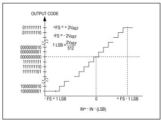
Figure 5. Bipolar Transfer Function
