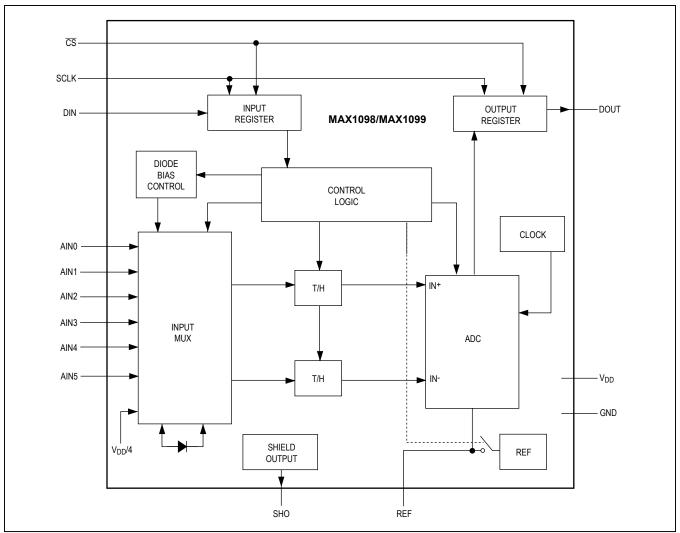
Figure 1. MAX1098/MAX1099 Functional Diagram
