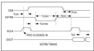
Figure 6. Detailed SSTRB Timing
