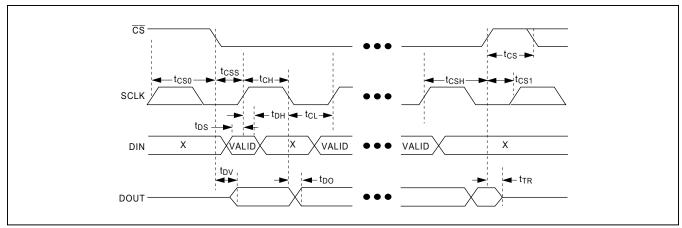
Figure 4. Detailed Serial Interface Timing
