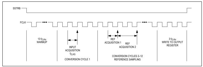
Figure 3a. Voltage Conversion Timing Diagram
