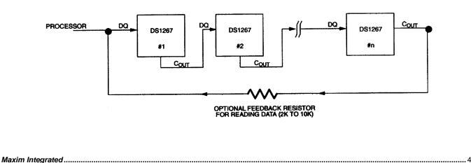
The C<sub>OUT</sub> output of the DS1267B can be used to drive the DQ input of another DS1267B. When connecting multiple devices, the total number of bits transmitted is always 17 times the number of DS1267Bs in the daisy chain.
