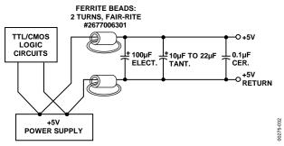
Figure 32. Single-Supply Analog Supply Filter
