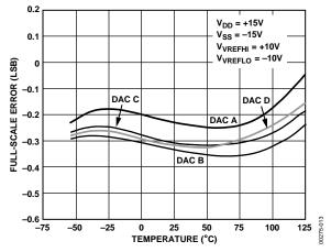
Figure 12. Full-Scale Error vs. Temperature
