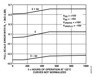
Figure 10. Full-Scale Error vs. Time Accelerated by Burn-In
