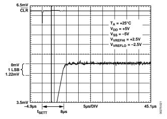
Figure 20. Negative Settling Time (±5 V)
