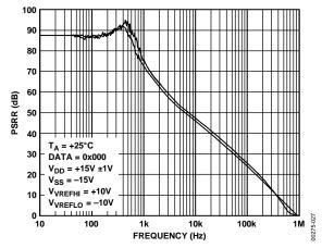
Figure 26. PSRR vs. Frequency
