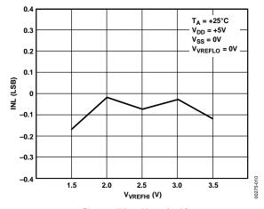
Figure 9. INL vs. V<sub>VREFHI</sub> (+5 V)
