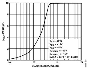
Figure 29. Output Swing vs. Load Resistance
