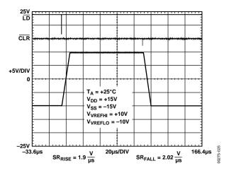
Figure 24. Slew Rate (±15 V)
