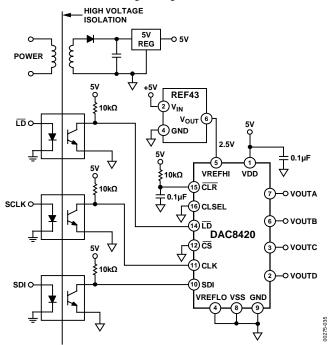
Figure 35. Opto-Isolated 3-Wire Interface
