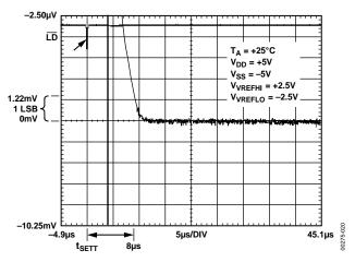
Figure 19. Positive Settling Time (±5 V)
