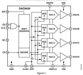
The user-programmable reset control  $\overline{\text{CLR}}$  forces all four DAC outputs to either zero scale or midscale, asynchronously overriding the current DAC register values. The output voltage range, determined by the inputs VREFHI and VREFLO, is set by the user for positive or negative unipolar or bipolar signal swings within the supplies, allowing considerable design flexibility.
