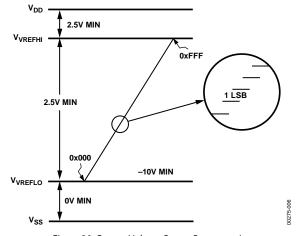
Figure 30. Output Voltage Range Programming
