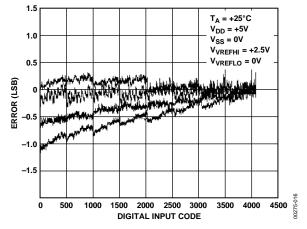
Figure 15. Channel-to-Channel Matching
