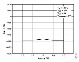
Figure 7. DNL vs. V<sub>VREFHI</sub> (+5 V)
