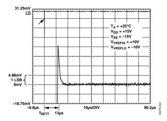
Figure 21. Positive Settling Time (±15 V)
