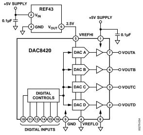
Figure 34. 5 V Single-Supply Operation Using REF43
