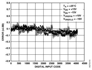
Figure 14. Channel-to-Channel Matching
