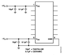
Figure 31. Recommended Supply Bypassing Scheme
