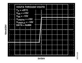
Figure 28. DAC Output Current vs. VOUTx
