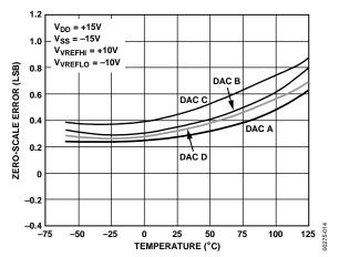
Figure 13. Zero-Scale Error vs. Temperature
