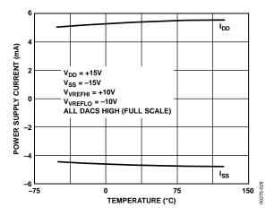
Figure 27. Power Supply Current vs. Temperature
