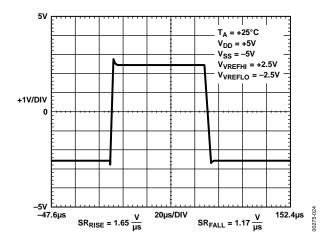
Figure 23. Slew Rate (±5 V)
