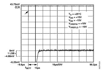
Figure 22. Negative Settling Time (±15 V)
