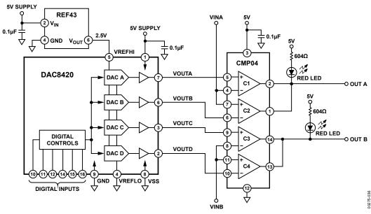
Figure 36. Dual Programmable Window Comparator
