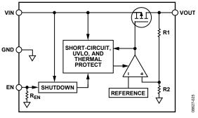
Figure 27. Internal Block Diagram
