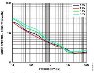
Figure 23. Output Noise Spectral Density vs. Frequency,  $V_{IN} = 5 V$ ,  $I_{LOAD} = 10 \text{ mA}$ ,  $C_{OUT} = 1 \mu F$
