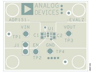
Figure 62. Example LFCSP PCB Layout
