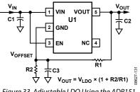
Figure 33. Adjustable LDO Using the ADP151
