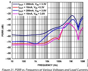
Figure 21. PSRR vs. Frequency at Various Voltages and Load Currents,  $V_{\rm OUT}$  = 2.8 V
