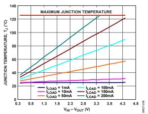
Figure 46. TSOT 100 mm<sup>2</sup> of PCB Copper,  $T_A = 25^{\circ}C$
