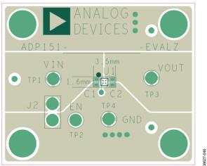
Figure 61. Example WLCSP PCB Layout
