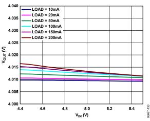
Figure 35. 4 V LDO Circuit, Typical Line Regulation over Load Current
