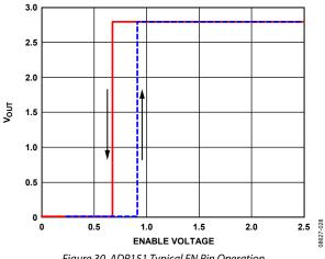
Figure 30. ADP151 Typical EN Pin Operation
