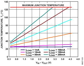
Figure 41. WLCSP 50 mm<sup>2</sup> of PCB Copper,  $T_A = 25^{\circ}C$
