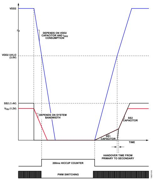
Figure 20. Remote Software Reset with 200 ms Hiccup
