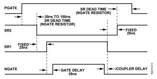
Figure 17. Gate Delay and SR Dead Time Settings
