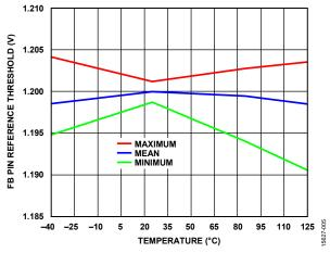
Figure 8. FB Pin Reference Threshold vs. Temperature
