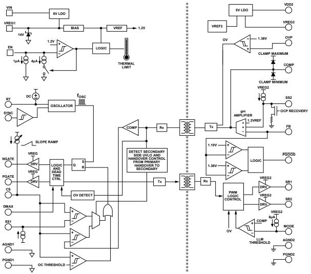
Figure 13. Detailed Block Diagram
