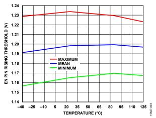
Figure 6. EN Pin Rising Threshold vs. Temperature
