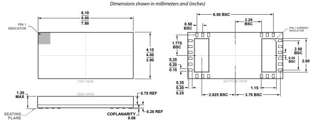
Figure 29. 24-Terminal Land Grid Array [LGA] (CC-24-6) Dimensions shown in millimeters
