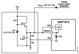
Figure 19. Fast Start-Up Circuit
