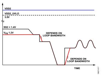
Figure 21. Tracking with SS2 Pin
