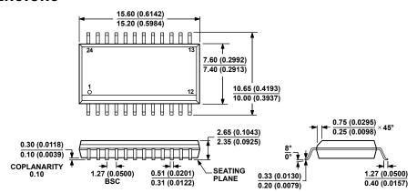
COMPLIANT TO JEDEC STANDARDS MS-013-AD CONTROLLING DIMENSIONS ARE IN MILLIMETERS; INCH DIMENSIONS (IN PARENTHESES) ARE ROUNDED-OFF MILLIMETER EQUIVALENTS FOR REFERENCE ONLY AND ARE NOT APPROPRIATE FOR USE IN DESIGN.
