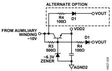
Figure 15. Recommended Circuit to Guarantee Hiccup Mode Showing
