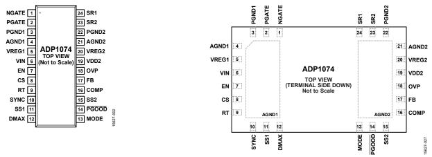
Figure 4. 24-Lead SOIC\_W Pin Configuration
