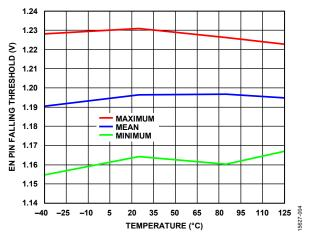
Figure 7. EN Pin Falling Threshold vs. Temperature
