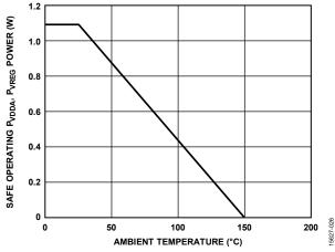
$Figure\ 2.\ Thermal\ Derative\ Curve,\ Dependence\ of\ Safety\ Limiting\ Values\ with\ Ambient\ Temperature\ per\ DINV\ VDE\ V\ 0884-10$
