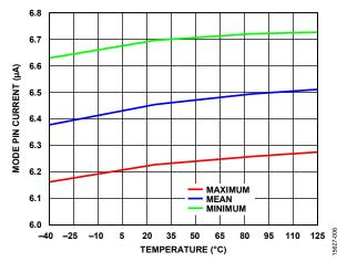
Figure 9. MODE Pin Current vs. Temperature
