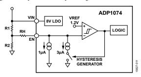
Figure 14. Precision EN with Adjustable Hysteresis
