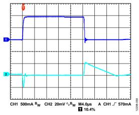
Figure 56. Output Transient Response,  $V_{OUT} = 5 V$ ,  $C_{OUT} = 4.7 \mu F$
