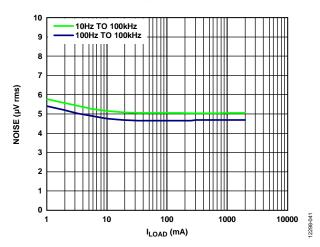
Figure 41. RMS Output Noise vs. Load Current (ILOAD), VOUT = 3 V
