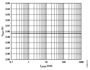
Figure 15. Output Voltage (VOUT) vs. Load Current (ILOAD), VOUT = 3 V
