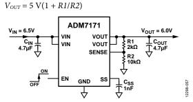
Figure 55. Typical Adjustable Output Voltage Application Schematic
