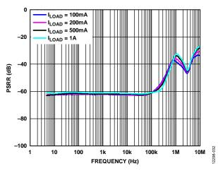
Figure 32. Power Supply Rejection Ratio (PSRR) vs. Frequency, 800 mV Headroom, V<sub>OUT</sub> = 3 V
