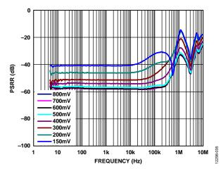
Figure 35. Power Supply Rejection Ratio (PSRR) vs. Frequency,  $V_{OUT} = 5 V$ , 1 A Load Current, Various Headroom Voltages
