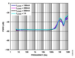
Figure 38. Power Supply Rejection Ratio (PSRR) vs. Frequency, 400 mV Headroom, V<sub>OUT</sub> = 5 V
