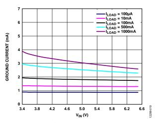
Figure 19. Ground Current vs. Input Voltage ( $V_{IN}$ ),  $V_{OUT} = 3 V$
