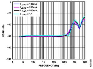
Figure 33. Power Supply Rejection Ratio (PSRR) vs. Frequency, 400 mV Headroom, V<sub>OUT</sub> = 3 V
