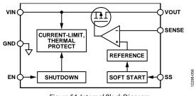
Figure 54. Internal Block Diagram
