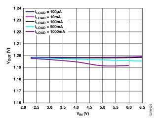
Figure 25. Output Voltage (V<sub>OUT</sub>) vs. Input Voltage (V<sub>IN</sub>), Adjustable Version,  $V_{OUT} = 1.2 V$
