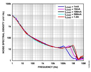
Figure 45. Output Noise Spectral Density,  $V_{OUT} = 3 V$
