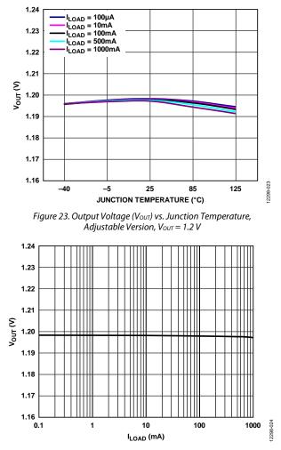
Figure 24. Output Voltage (V<sub>OUT</sub>) vs. Load Current ( $I_{LOAD}$ ), Adjustable Version, V<sub>OUT</sub> = 1.2 V
