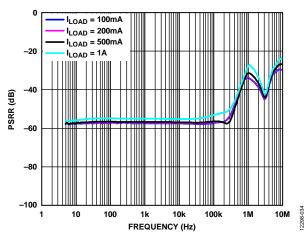
Figure 34. Power Supply Rejection Ratio (PSRR) vs. Frequency, 300 mV Headroom, V<sub>OUT</sub> = 3 V
