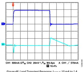
Figure 48. Load Transient Response,  $I_{LOAD} = 10$  mA to 1 A,  $V_{OUT} = 5$  V,  $V_{IN} = 5.5$  V, CH1 =  $I_{LOAD}$ , CH2 =  $V_{OUT}$
