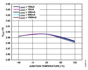
Figure 14. Output Voltage ( $V_{OUT}$ ) vs. Junction Temperature,  $V_{OUT}$  = 3 V
