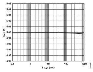
Figure 5. Output Voltage (Vout) vs. Load Current (ILOAD)
