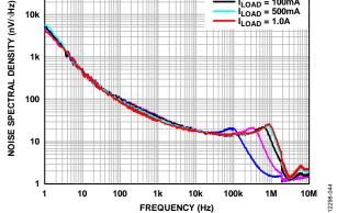
Figure 44. Output Noise Spectral Density, Adjustable Version, Vout = 1.2 V
