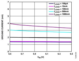
Figure 9. Ground Current vs. Input Voltage (VIN)
