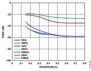
Figure 36. Power Supply Rejection Ratio (PSRR) vs. Headroom,  $V_{OUT} = 5 V$ , 1 A Load Current, Different Frequencies
