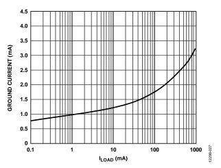
Figure 27. Ground Current vs. Load Current (I<sub>LOAD</sub>), Adjustable Version,  $V_{OUT} = 1.2 V$
