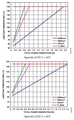
In the case where the board temperature is known, use the thermal characterization parameter,  $\Psi_{JB}$ , to estimate the junction temperature rise. Maximum junction temperature (T<sub>J</sub>) is calculated from the board temperature (T<sub>B</sub>) and power dissipation (P<sub>D</sub>) using the following formula:
