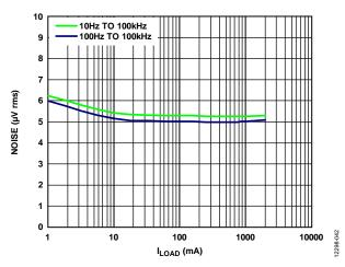
Figure 42. RMS Output Noise vs. Load Current (ILOAD), VOUT = 5 V
