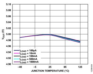
Figure 4. Output Voltage ( $V_{OUT}$ ) vs. Junction Temperature
