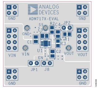
Figure 69. Example LFCSP PCB Layout
