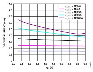
Figure 28. Ground Current vs. Input Voltage (V<sub>N</sub>), Adjustable Version,  $V_{OUT} = 1.2 V$
