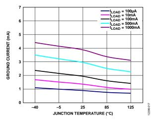
Figure 17. Ground Current vs. Junction Temperature,  $V_{OUT} = 3 V$
