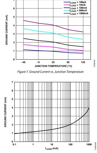
Figure 8. Ground Current vs. Load Current (ILOAD)
