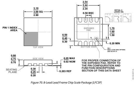
Figure 70. 8-Lead Lead Frame Chip Scale Package [LFCSP] 3 mm × 3 mm Body and 0.75 mm Package Height (CP-8-21) Dimensions shown in millimeters
