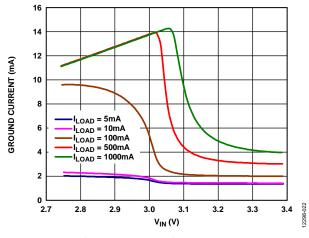
Figure 22. Ground Current vs. Input Voltage ( $V_{IN}$ ) in Dropout,  $V_{OUT} = 3 V$
