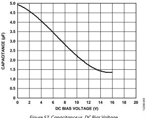
Figure 57. Capacitance vs. DC Bias Voltage
