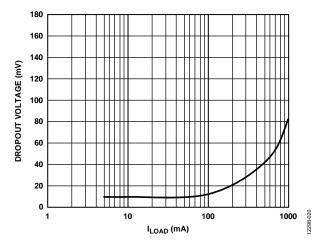
Figure 20. Dropout Voltage vs. Load Current (ILOAD), VOUT = 3 V
