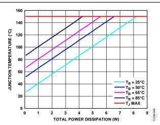
Figure 66. LFCSP Power Dissipation for Various Board Temperatures
