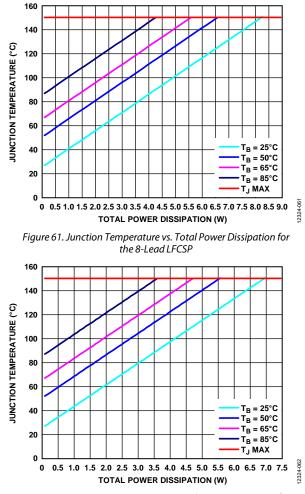
Figure 62. Junction Temperature vs. Total Power Dissipation for the 8-Lead SOIC
