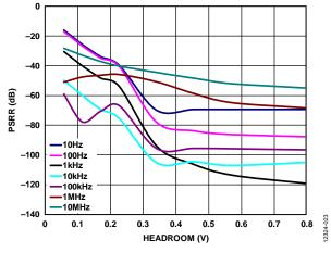
Figure 23. Power Supply Rejection Ratio (PSRR) vs. Headroom Voltage at Different Frequencies, Vout = 3.3 V, 400 mA Load
