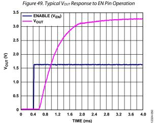
Figure 50. Typical V<sub>OUT</sub> Response to EN Pin Operation (V<sub>EN</sub>),  $V_{OUT} = 3.3 V$ ,  $V_{IN} = 5 V$ ,  $C_{BYP} = 1 \mu F$
