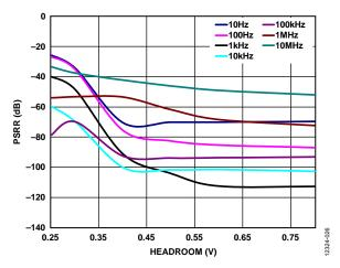
Figure 26. Power Supply Rejection Ratio (PSRR) vs. Headroom Voltage, Different Frequencies, Vout = 1.8 V, 400 mA Load
