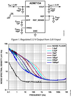
Figure 2. Noise Spectral Density for Different Values of CBYP
