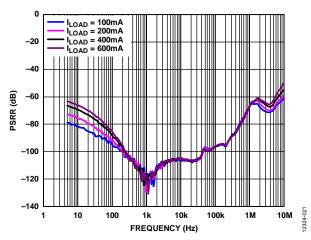
Figure 21. Power Supply Rejection Ratio (PSRR) vs. Frequency at Various Loads,  $V_{OUT}$  = 3.3 V,  $V_{IN}$  = 4.1 V
