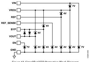
Figure 43. Simplified ESD Protection Block Diagram
