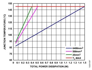
Figure 57. Junction Temperature vs. Total Power Dissipation for the 8-Lead LFCSP,  $T_A = 85^{\circ}C$
