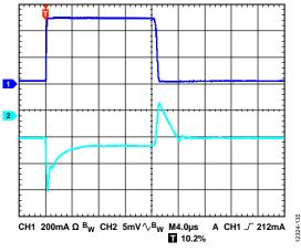
Figure 35. Load Transient Response, I<sub>LOAD</sub> = 10 mA to 510 mA, V<sub>OUT</sub> = 3.3 V, V<sub>IN</sub> = 3.8 V, CH1 = I<sub>OUT</sub>, CH2 = V<sub>OUT</sub>
