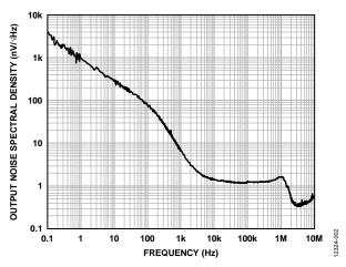
Figure 32. Output Noise Spectral Density, 0.1 Hz to 10 MHz, ILOAD = 100 mA
