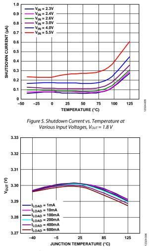
Figure 6. Output Voltage ( $V_{OUT}$ ) vs. Junction Temperature at Various Loads,  $V_{OUT} = 3.3 V$
