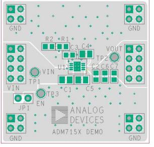
Figure 63. Example 8-Lead LFCSP PCB Layout
