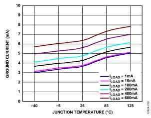
Figure 18. Ground Current vs. Junction Temperature (T\_J) at Various Loads,  $V_{OUT} = 1.8 V$
