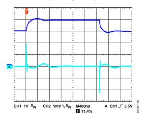
Figure 40. Line Transient Response, 1 V Input Step, I<sub>LOAD</sub> = 600 mA, V<sub>OUT</sub> = 1.8 V, V<sub>IN</sub> = 2.4 V, CH1 = V<sub>IN</sub>, CH2 = V<sub>OUT</sub>
