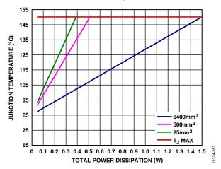
Figure 58. Junction Temperature vs. Total Power Dissipation for the 8-Lead SOIC,  $T_A = 25^{\circ}C$
