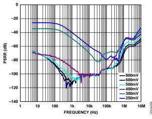
Figure 25. Power Supply Rejection Ratio (PSRR) vs. Frequency at Various Headroom Voltages, Vout = 1.8 V, 400 mA Load
