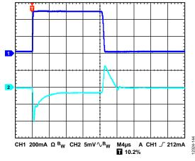
Figure 44. Output Transient Response,  $V_{OUT} = 3.3 V$ ,  $C_{OUT} = 10 \mu F$ , CH1 = Load Current, CH2 =  $V_{OUT}$
