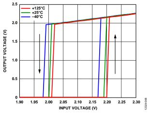
Figure 48. Typical UVLO Behavior at Different Temperatures,  $V_{OUT} = 3.3 V$
