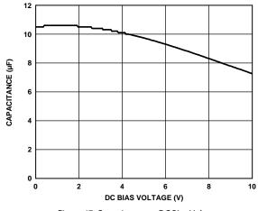
Figure 47. Capacitance vs. DC Bias Voltage
