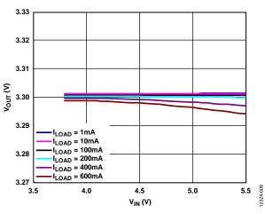
Figure 8. Output Voltage ( $V_{OUT}$ ) vs. Input Voltage ( $V_{IN}$ ) at Various Loads,  $V_{OUT} = 3.3 V$
