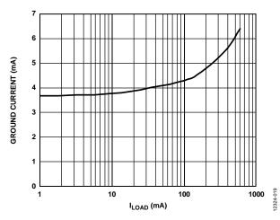
Figure 19. Ground Current vs. Load Current (ILOAD), VOUT = 1.8 V
