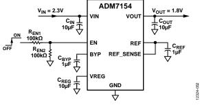
Figure 52. Typical EN Pin Voltage Divider
