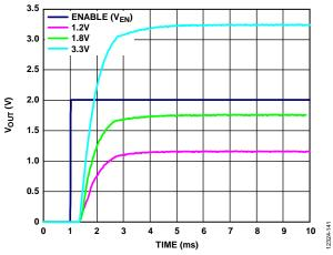
Figure 41. V<sub>OUT</sub> Start-Up Time After V<sub>EN</sub> Rising, Different Output Voltages,  $V_{\rm IN} = 5$  V
