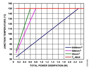
Figure 56. Junction Temperature vs. Total Power Dissipation for the 8-Lead LFCSP,  $T_A = 50^{\circ}$ C
