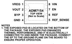
Figure 3. 8-Lead LFCSP Pin Configuration
