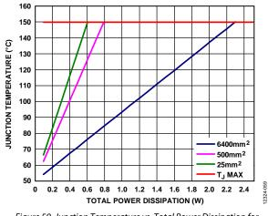
Figure 59. Junction Temperature vs. Total Power Dissipation for the 8-Lead SOIC,  $T_A = 50^{\circ}C$
