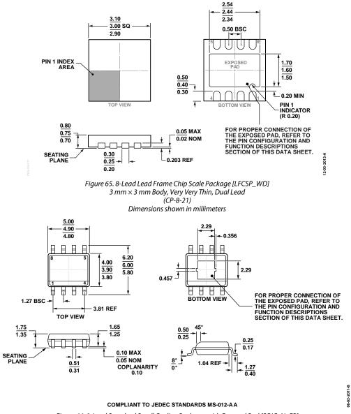
Figure 66. 8-Lead Standard Small Outline Package, with Exposed Pad [SOIC\_N\_EP] Narrow Body (RD-8-1) Dimensions shown in millimeters
