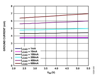
Figure 20. Ground Current vs. Input Voltage (V\_IN) at Different Loads,  $V_{OUT} = 1.8 V$
