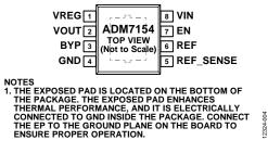
Figure 4. 8-Lead SOIC Pin Configuration
