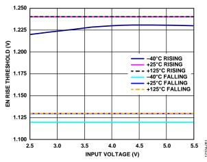
Figure 51. Typical EN Threshold vs. Input Voltages (V<sub>IN</sub>) for Different Temperatures
