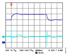
Figure 39. Line Transient Response, 1 V Input Step, I<sub>LOAD</sub> = 600 mA, V<sub>OUT</sub> = 3.3 V, V<sub>IN</sub> = 3.9 V, CH1 = V<sub>IN</sub>, CH2 = V<sub>OUT</sub>
