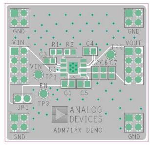
Figure 64. Example 8-Lead SOIC PCB Layout
