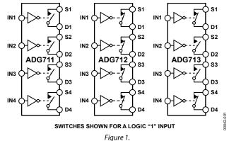
The ADG711/ADG712/ADG713 are available in 16-lead TSSOP and 16-lead SOIC packages.
