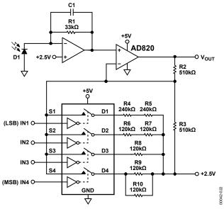
Figure 20. Photodetector Circuit with Programmable Gain
