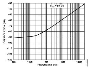
Figure 7. Off Isolation vs. Frequency
