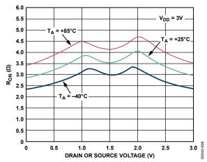
Figure 4. On Resistance as a Function of  $V_D$  (V<sub>s</sub>) for Different Temperatures  $V_{DD}$  = 3 V
