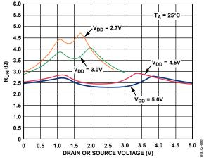
Figure 3. On Resistance as a Function of  $V_D$  (V<sub>S</sub>)
