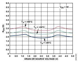
Figure 5. On Resistance as a Function of  $V_{\rm D}$  (Vs) for Different Temperatures  $V_{\rm DD}$  = 5 V
