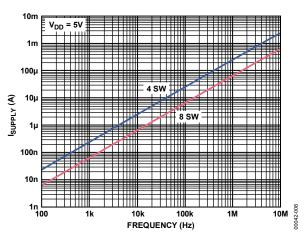
Figure 6. Supply Current vs. Input Switching Frequency
