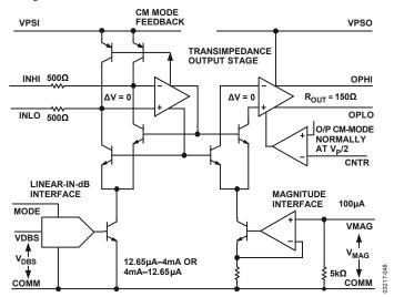
Figure 47. Schematic of Key Components
