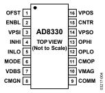
Figure 3. 16-Lead QSOP Pin Configuration
