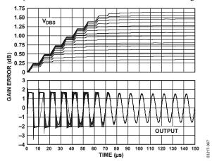
Figure 66. Time Domain Waveforms (Simulation)
