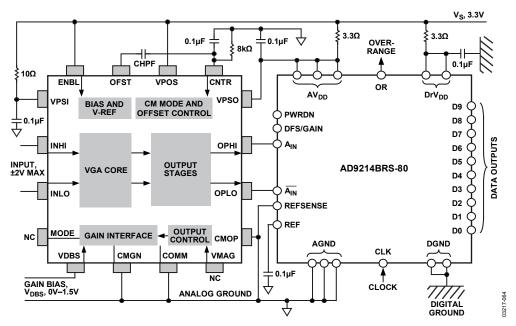
Figure 63. Driving an Analog-to-Digital Converter (Preliminary)
