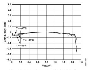
Figure 6. Gain Linearity Error Normalized at 25°C vs.  $V_{DBS}$ , at Three Temperatures, f = 1 MHz
