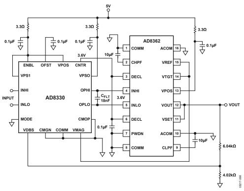
Figure 67. Wide Range True RMS Voltmeter (Preliminary)
