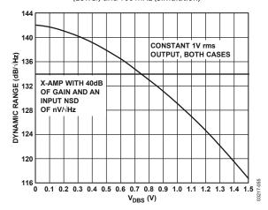
Figure 54. Dynamic Range in dB/ $\sqrt{Hz}$  vs.  $V_{DBS}$  ( $V_{MAG} = 0.5 V$ , 1 V rms Output) Compared with a Representative X-AMP (Simulation)
