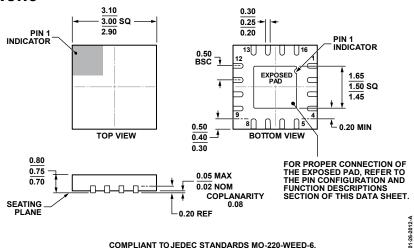
Figure 78. 16-Lead Lead Frame Chip Scale Package [LFCSP] 3 mm × 3 mm Body and 0.75 mm Package Height
