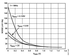
Figure 21. Input Referred Noise vs.  $V_{DBS}$  for Three Values of  $V_{MAG}$
