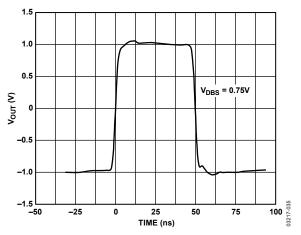
Figure 34. Full-Scale Transient Response,  $V_{DBS} = 0.75 V$ , f = 1 MHz,  $V_{OUT} = 2 V p$ -p
