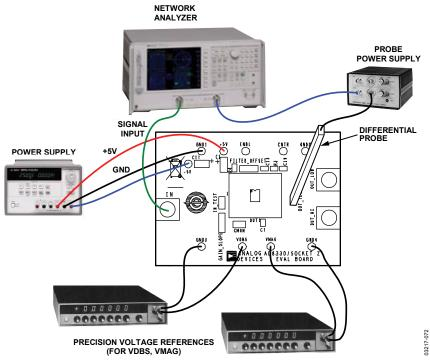
Figure 71. Typical Connections
