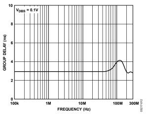
Figure 11. Group Delay vs. Frequency
