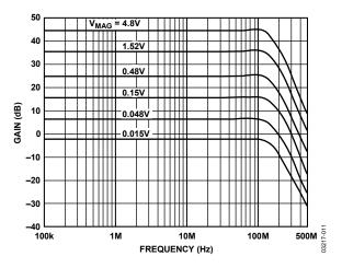
Figure 10. Frequency Response for Various Values of  $V_{MAG_r}$  $V_{DBS} = 0.75 V$
