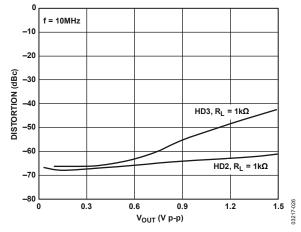
Figure 25. Harmonic Distortion vs.  $V_{OUT}$ ,  $V_{MAG} = 0.5 V$
