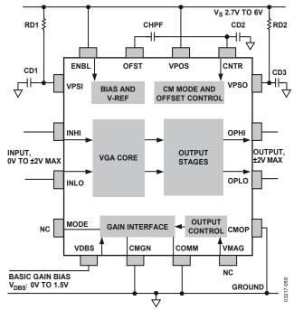
Figure 57. Power Supply Decoupling and Basic Connections
