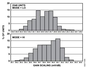
Figure 8. Gain Slope Histogram
