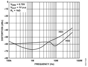
Figure 23. Harmonic Distortion vs. Frequency
