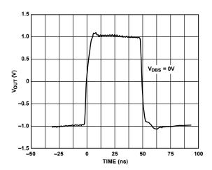
Figure 33. Full-Scale Transient Response,  $V_{DBS} = 0 V$
