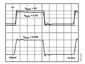
Figure 39. Transient Response vs. V<sub>MAG</sub>
