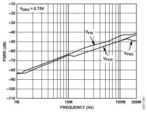
Figure 42. PSRR vs. Frequency
