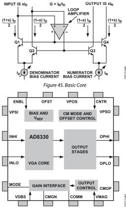
Figure 46. Block Schematic
