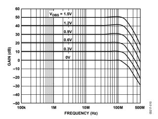
Figure 9. Frequency Response in 10 dB Steps for Various Values of  $V_{\text{DBS}}$
