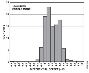
Figure 13. Differential Input Offset Histogram
