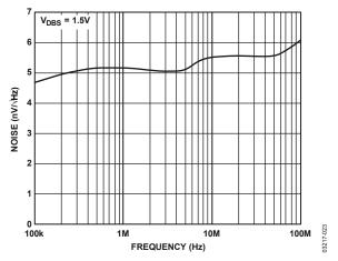
Figure 22. Input Referred Noise vs. Frequency
