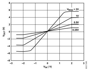
Figure 49. Effect of V<sub>MAG</sub> on Gain and Peak Output
