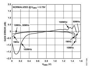
Figure 7. Gain Error vs. V<sub>DBS</sub> at Various Frequencies
