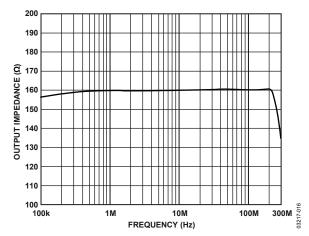
Figure 15. Output Impedance vs. Frequency
