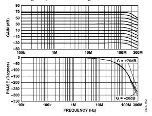
Figure 51. AC Performance over a 100 dB Gain Range Obtained by Using Two Values of V<sub>MAG</sub>
