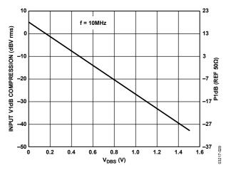
Figure 28. Input V1dB Compression vs. VDBS
