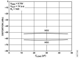
Figure 24. Harmonic Distortion vs. CLOAD
