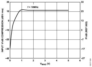
Figure 29. Output V1dB Compression vs. V<sub>MAG</sub>
