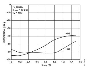
Figure 27. Harmonic Distortion vs. V<sub>DBS</sub>
