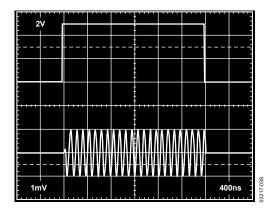
Figure 38. V<sub>MAG</sub> Interface Response, Top: V<sub>MAG</sub>, Bottom: V<sub>OUT</sub>
