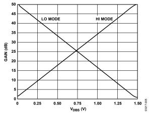
Figure 4. Gain vs. V<sub>DBS</sub>
