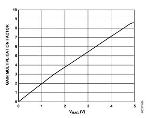
Figure 5. Linear Gain Multiplication Factor vs. V<sub>MAG</sub>
