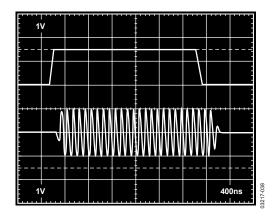
Figure 37. V<sub>DBS</sub> Interface Response, Top: V<sub>DBS</sub>, Bottom: V<sub>OUT</sub>
