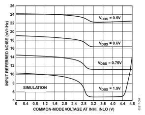
Figure 56. Input Noise vs. Common-Mode Input Voltage for  $V_{DBS} = 0.5 \text{ V}$ , 0.6 V, 0.75 V, and 1.5 V
