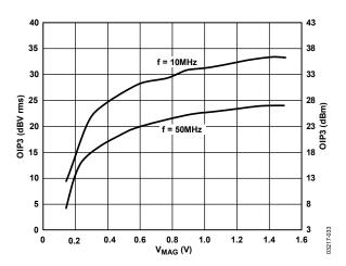
Figure 32. OIP3 vs. V<sub>MAG</sub>
