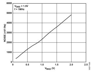
Figure 19. Output Referred Noise vs. V<sub>MAG</sub>
