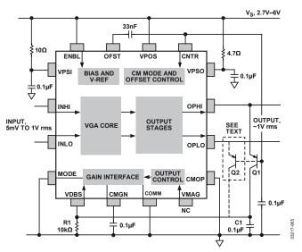
Figure 64. Simple AGC Amplifier (Preliminary)
