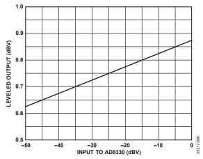
Figure 65. AGC Output vs. Input Amplitude (Simulation)
