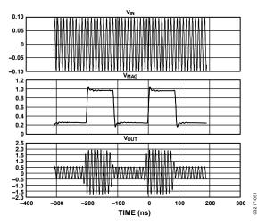
Figure 50. Using VMAG in Modulation Mode
