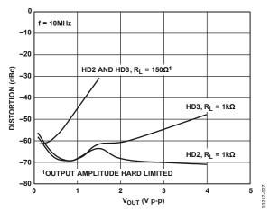
Figure 26. Harmonic Distortion vs.  $V_{OUT}$ ,  $V_{MAG} = 2.0 V$
