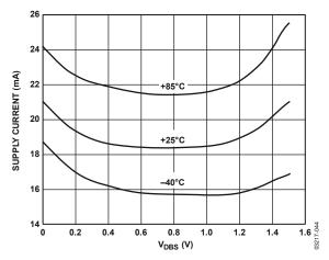
Figure 43. Supply Current vs.  $V_{DBS}$  at Three Temperatures
