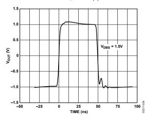
Figure 35. Full-Scale Transient Response,  $V_{DBS} = 1.5 \text{ V}$ , f = 1 MHz,  $V_{OUT} = 2 \text{ V } p\text{-}p$
