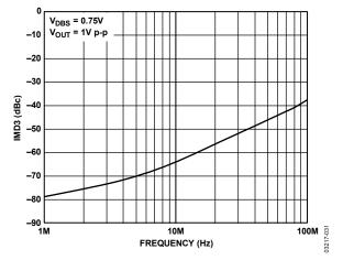
Figure 30. IMD3 Distortion vs. Frequency
