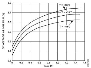
Figure 55. Common-Mode Voltage at Input Pins vs.  $V_{DBS}$ , for  $V_S = 5 V$ ,  $T = -40^{\circ}\text{C}$ ,  $+25^{\circ}\text{C}$ , and  $+85^{\circ}\text{C}$
