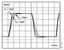
Figure 36. Transient Response vs. Various Load Capacitances, G = 25 dB
