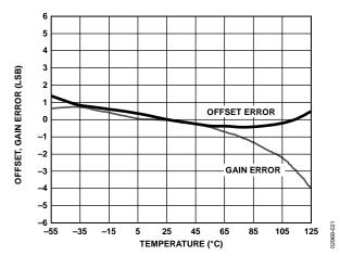
Figure 23. Offset and Gain Error vs. Temperature
