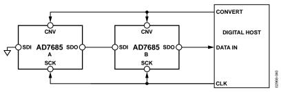
Figure 42. Chain Mode Connection Diagram
