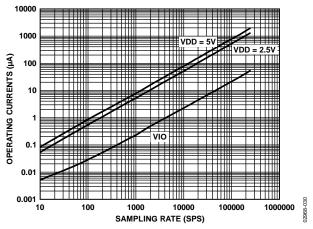
Figure 32. Operating Currents vs. Sampling Rate
