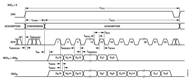
Figure 43. Chain Mode Serial Interface Timing
