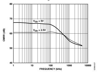
Figure 29. Analog Input CMRR vs. Frequency
