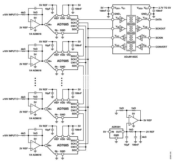
Figure 48. A True 16-Bit Isolated Simultaneous Sampling Acquisition System
