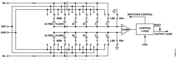
Figure 25. ADC Simplified Schematic
