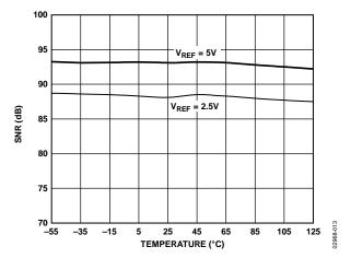
Figure 15. SNR vs. Temperature
