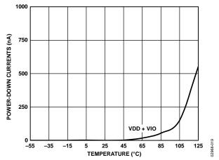
Figure 21. Power-Down Currents vs. Temperature
