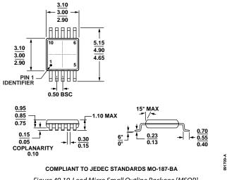
Figure 49.10-Lead Micro Small Outline Package [MSOP] (RM-10) Dimensions shown in millimeters
