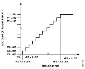
Figure 26. ADC Ideal Transfer Function
