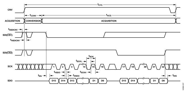
Figure 39. CS Mode 4-Wire, No BUSY Indicator Serial Interface Timing
