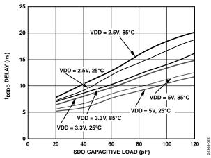
Figure 24. t<sub>DSDO</sub> Delay vs. Capacitance Load and Supply
