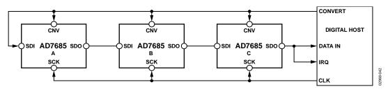
Figure 44. Chain Mode with BUSY Indicator Connection Diagram
