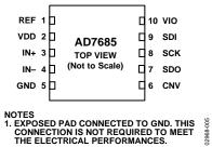
Figure 6. 10-Lead LFCSP Pin Configuration
