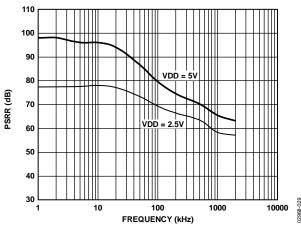
Figure 31. PSRR vs. Frequency
