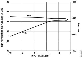
Figure 19. SNR and THD vs. Input Level
