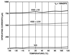
Figure 22. Operating Currents vs. Temperature
