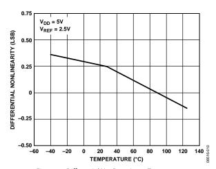
Figure 11. Differential Nonlinearity vs. Temperature
