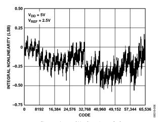
Figure 7. Integral Nonlinearity vs. Code
