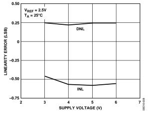
Figure 9. Linearity Error vs. Supply Voltage
