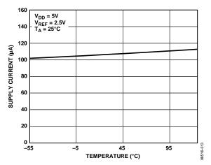
Figure 14. Supply Current vs. Temperature
