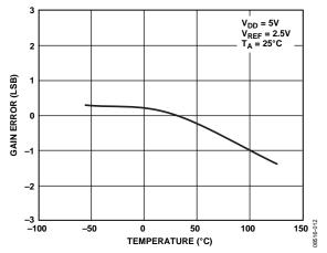
Figure 13. Gain Error vs. Temperature
