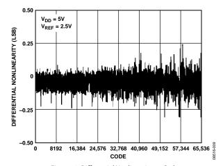
Figure 10. Differential Nonlinearity vs. Code
