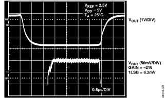
Figure 22. Small Signal Settling Time
