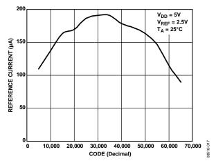
Figure 18. Reference Current vs. Code
