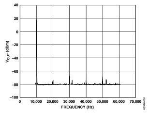
Figure 28. Total Harmonic Distortion
