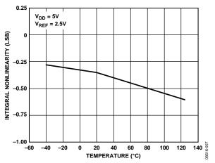
Figure 8. Integral Nonlinearity vs. Temperature
