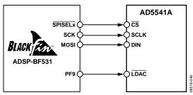
Figure 32. AD5541A to ADSP-BF531 Interface
