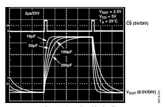
Figure 21. Large Signal Settling Time
