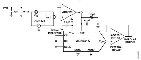
Figure 31. Unipolar Output
