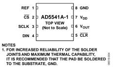
Figure 5. AD5541A-1 8-Lead LFCSP Pin Configuration
