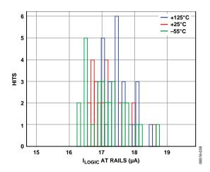
Figure 24. Digital Supply Current Histogram
