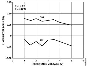
Figure 12. Linearity Error vs. Reference Voltage
