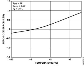
Figure 16. Zero-Code Error vs. Temperature
