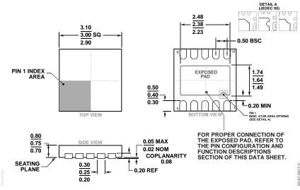
Figure 37. 10-Lead Lead Frame Chip Scale Package [LFCSP] 3 mm × 3 mm Body and 0.75 mm Package Height (CP-10-9) Dimensions shown in millimeters
