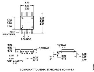
Figure 36. 10-Lead Mini Small Outline Package [MSOP] (RM-10) Dimensions shown in millimeters
