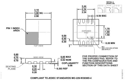
Figure 38. 8-Lead Lead Frame Chip Scale Package [LFCSP] 3 mm × 3 mm Body and 0.75 mm Package Height (CP-8-11) Dimensions shown in millimeters
