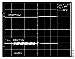
Figure 19. Digital Feedthrough
