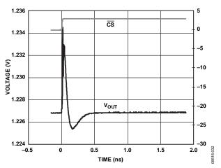
Figure 20. Digital-to-Analog Glitch Impulse
