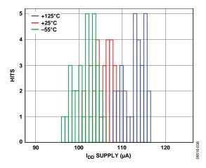
Figure 23. Analog Supply Current Histogram
