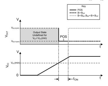
Figure 3: Power-On Sequence and Timing
