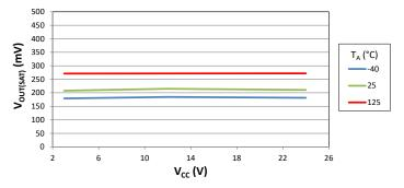
Average Low Output Voltage versus Ambient Temperature for  $\rm I_{OUT}$  = 20 mA
