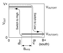
Figure 2: Device Switching Behavior
